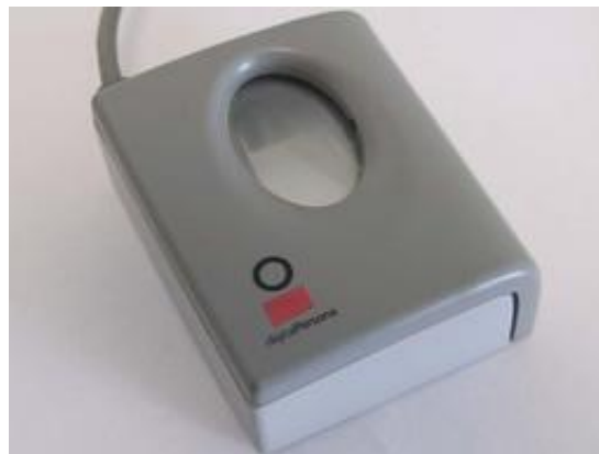
Figure 1: DigitalPersona's U.are.U scanner [8]
