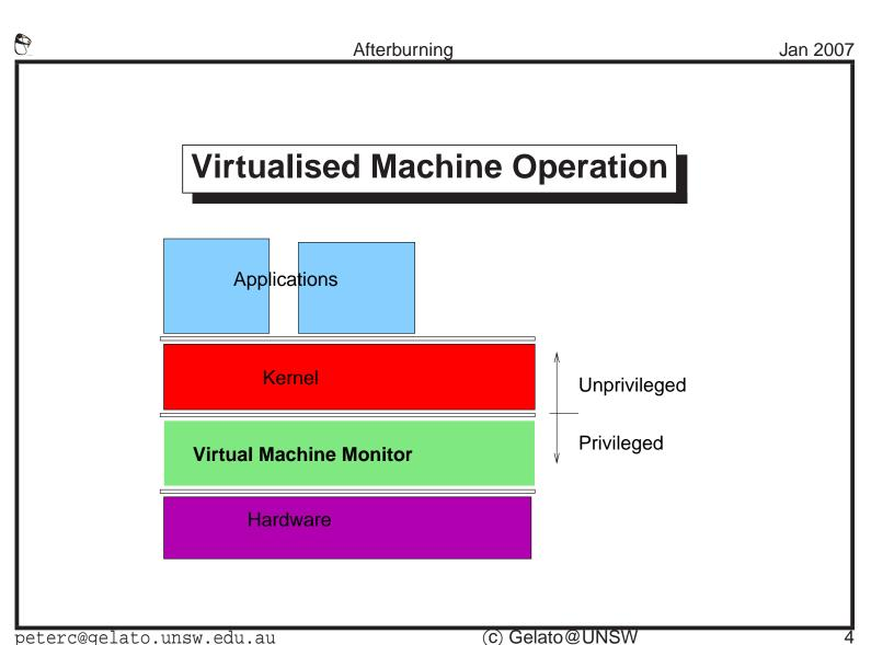
One approach used is to deprivilege the operating system kernel. Then when the kernel tries to do something special (like talk to the hardware), its attempt is trapped into a *Virtual Machine Monitor* (VMM), *supervisor* or *Hypervisor*. The VMM pretends to be a machine that looks more-or-less like the real one, while controlling page table, direct device and privileged system control register accesses.
