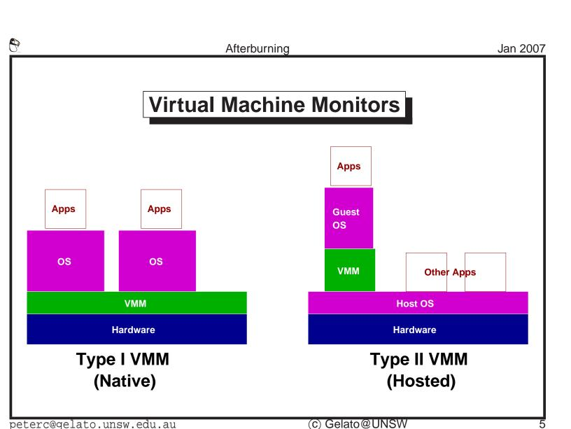
There are two kinds of virtual machine monitors (VMM). A *Type I* VMM controls the hardware directly (The nomenclature was originally introduced by [Goldberg, 1973]). Guest operating systems see a virtualised version of the hardware. Xen [Barham et al., 2003] and vNUMA [Chapman and Heiser, 2005] are examples of Type I VMMs.
