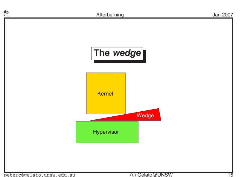
Having rewritten the code, there's still need to interface with a variety of hypervisors. This is done by means of a *wedge*, a piece of code that can be called by the rewritten code to interface into the hypervisor.
